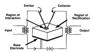
Fig. 3. Schematic diagram of the first transistor.
