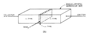
Fig. 4. The first junction transistor.
