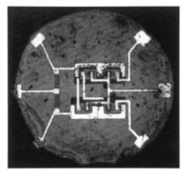
Fig. 7. Early Fairchild IC using planar process. (Reprinted by permission of Fairchild Semiconductor.)
