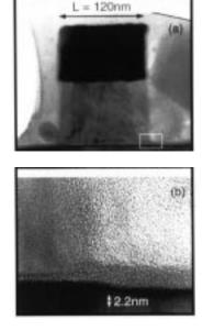
Fig. 9. Advanced FET cross section.
