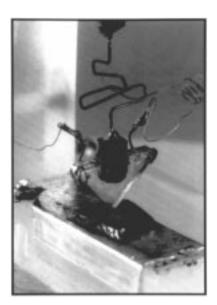
Fig. 2. The first transistor.
