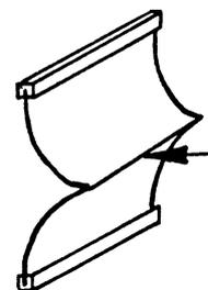
Figure 5.26: Diaphragm of a folded loudspeaker.
