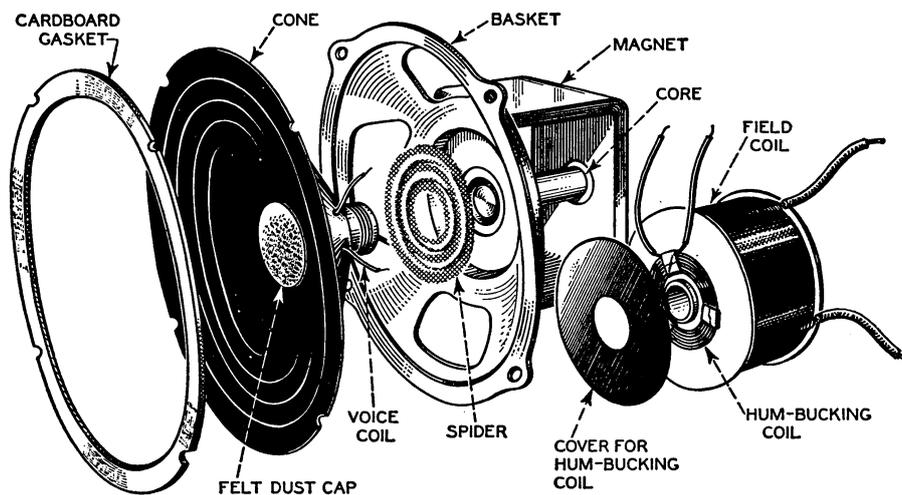
Figure 5.2: Exploded view of an electrodynamic loudspeaker
