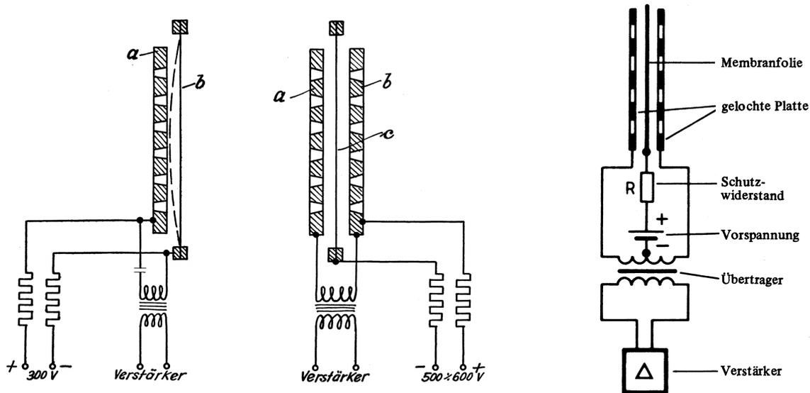
Figure 7.1: Principle of the electrostatic loudspeaker.
