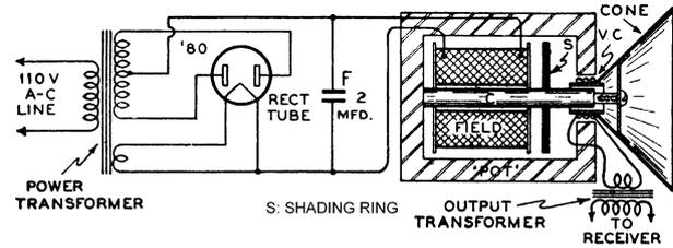
Figure 5.6: Electrodynamic loudspeaker with short-circuit field shading ring.
