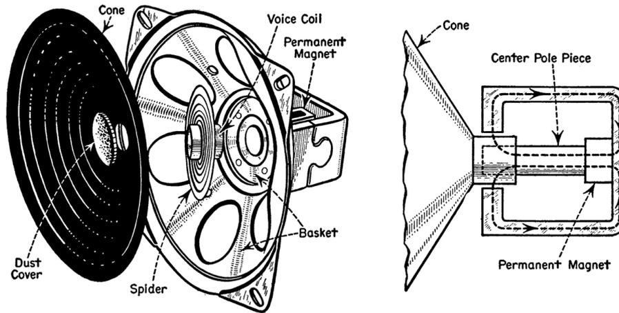
Figure 5.8: Exploded view of a permanent-magnet dynamic loudspeaker.
