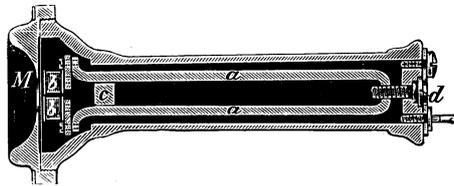
Figure 1.2: Telephone receiver with horse-shoe magnet shown in cross-section
