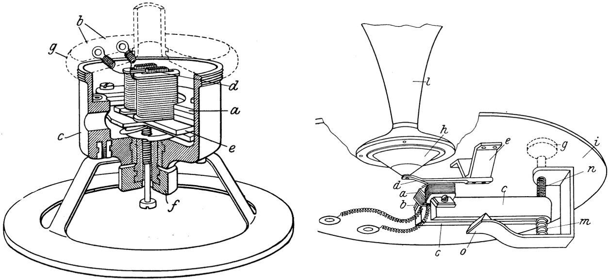
Figure 2.3: Examples of drive systems for horn-loudspeakers
