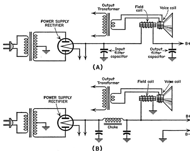
Figure 5.3: Field excitation of an electrodynamic loudspeaker: (A) Series-connection, (B) Parallel-connection.
