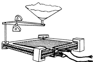
Figure 7.3: Drive system of saddle-bender.
