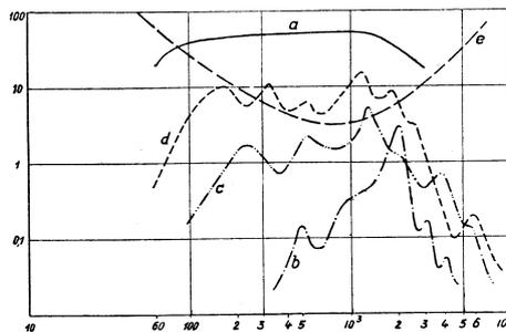
Figure 2.4: Typical loudspeaker frequency ranges: a) “ideal” b) ordinary horn c) Exponential horn d)dynamic loudspeaker in a baffle e)Ideal measured ear sensitivity.
