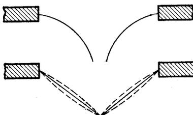
Figure 5.12: The NAWI diaphragm (above) as apposed to the cone shaped diaphragm, which can easily buckle (below).
