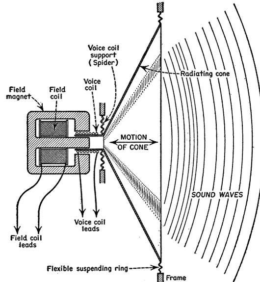
Figure 5.1: Cross-sectional view through an electrodynamic loudspeaker
