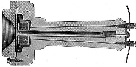
Figure 1.1: Bell receiver in cross-section
