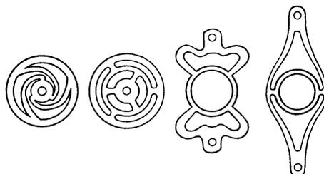
Figure 5.10: Older types of spiders for dynamic loudspeakers; on the right, two for internal mounting; on the left, two for external mounting.
