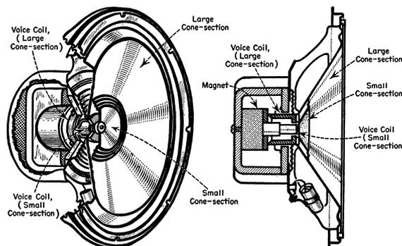
Figure 5.20: Woofer with built-in high frequency tweeter sharing different portions of the diaphragm. The two voice-coils are connected with a cross-over network.
