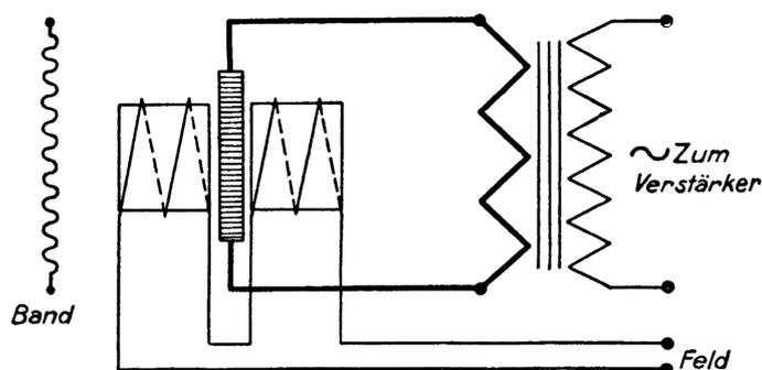
Figure 4.12: Principle of the Ribbon loudspeaker
