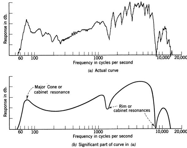
Figure 5.14: Example of the frequency response of a built-in speaker.
