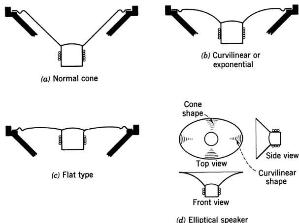
Figure 5.17: Typical diaphragm forms.
