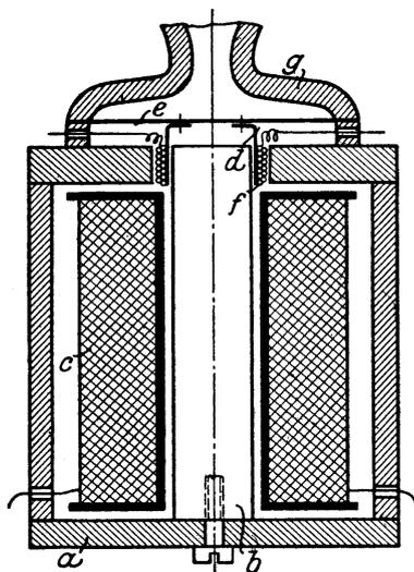
Figure 4.9: Cross-section of the Magnavox electrodynamic system.
