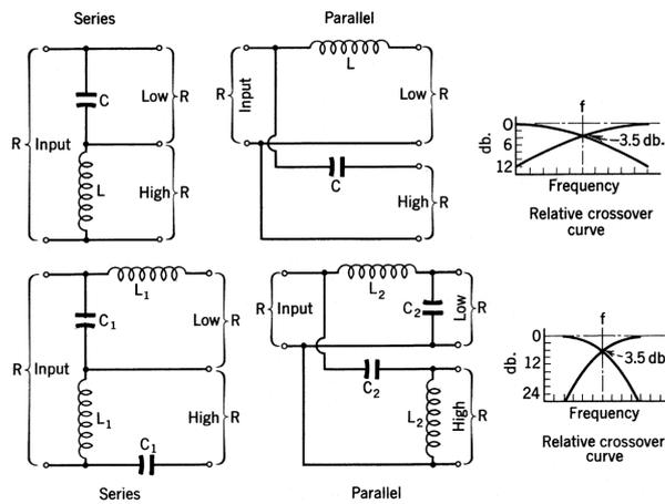
Figure 5.24: Single and two-pole and cross-over networks; series and parallel-connections.
