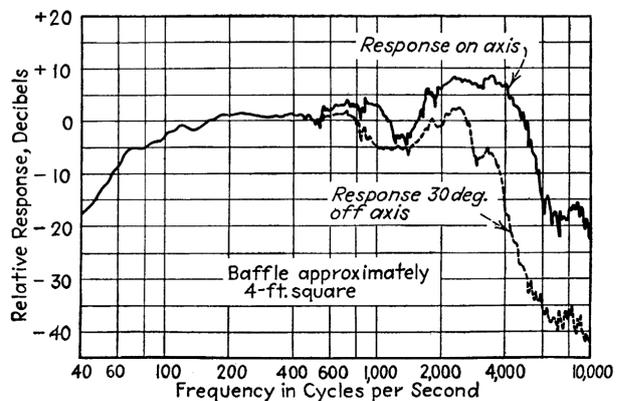
Figure 5.16: Angular dependence of the frequency response of a speaker in a baffle.
