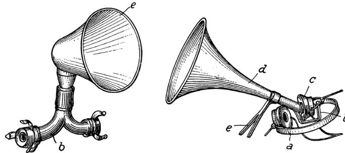
Figure 2.1: Coupling of earphones to horns: Left – for double headphones, right – improvised coupling to single transducer
