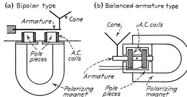
Figure 4.1: Drive systems for magnetic loudspeakers; left: steel reed anchored on a single end; right: unsprung balanced system.
