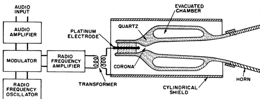
Figure 7.4: Principle of the ionic loudspeaker.
