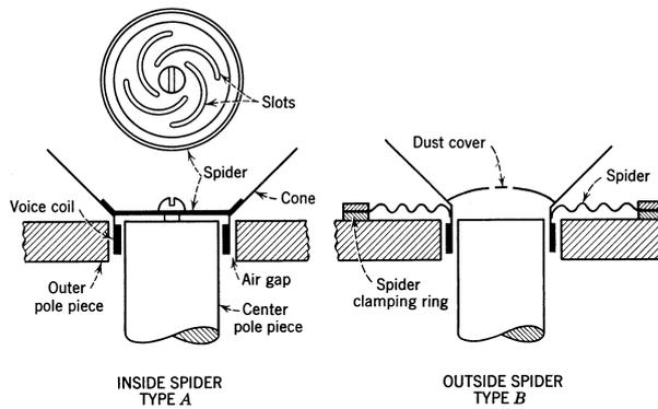
Figure 5.9: Inner centering spider of a dynamic loudspeaker; *A* internally mounted *B* externally mounted.
