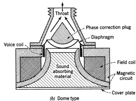
Figure 6.8: Drive system with inverse dome diaphragm.
