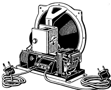
Figure 5.4: Electrodynamic loudspeaker with power supply for field excitation.
