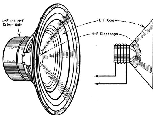
Figure 5.21: Woofer with high frequency dome.
