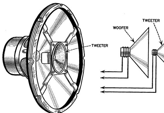
Figure 5.19: Combination of woofer with coaxial tweeter. The speakers are connected with a cross-over network.
