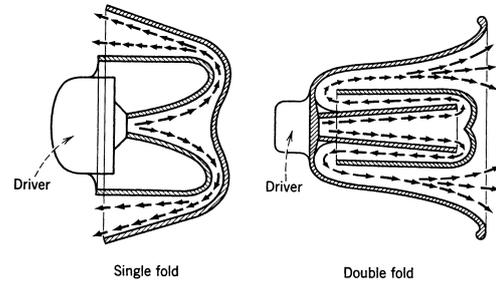
Figure 6.2: Modern folded horn-loudspeaker.
