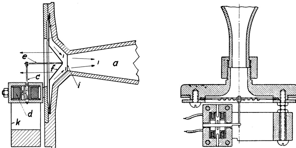
Figure 6.9: Four pole magnetic drive system in horn loudspeakers.
