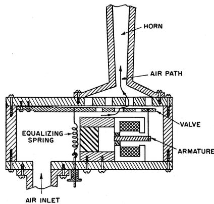
Figure 3.5: Pneumatic loudspeaker
