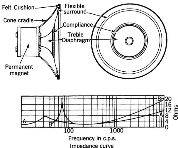
Figure 5.18: Wideband loudspeaker with subdivided diaphragm; impedance of the voice-coil (A) in comparison to a conventional loudspeaker (B).
