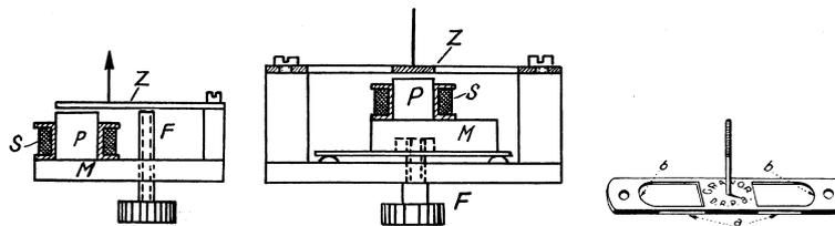
Figure 4.2: Reed system for magnetic loudspeakers; left: anchored on a single end; middle: anchored on two ends; right: steel reed detail *a* is damping material.
