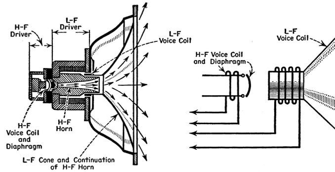
Figure 5.23: Coaxial speaker. The two voice-coils are connected with a cross-over network.
