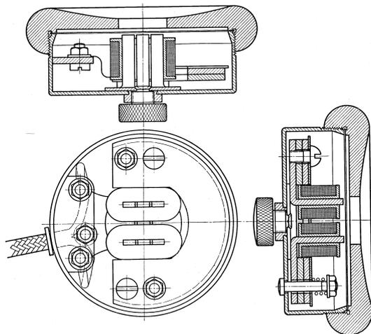
Figure 1.3: Headphone construction with adjustment for diaphragm distance.
