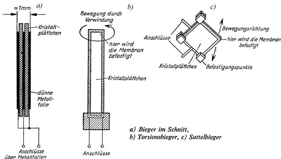
Figure 7.2: Drive system of a Crystal loudspeaker.
