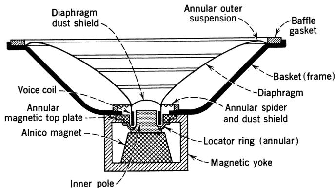
Note: Inexpensive speakers use magnetic yoke as magnetic top plate in single piece construction.
