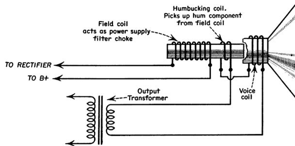
Figure 5.5: Electrodynamic loudspeaker with Hum-bucking.
