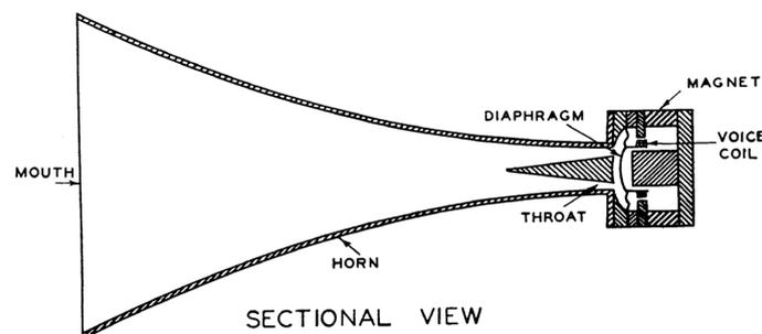
Figure 6.4: Cross-section of a horn-loudspeaker.
