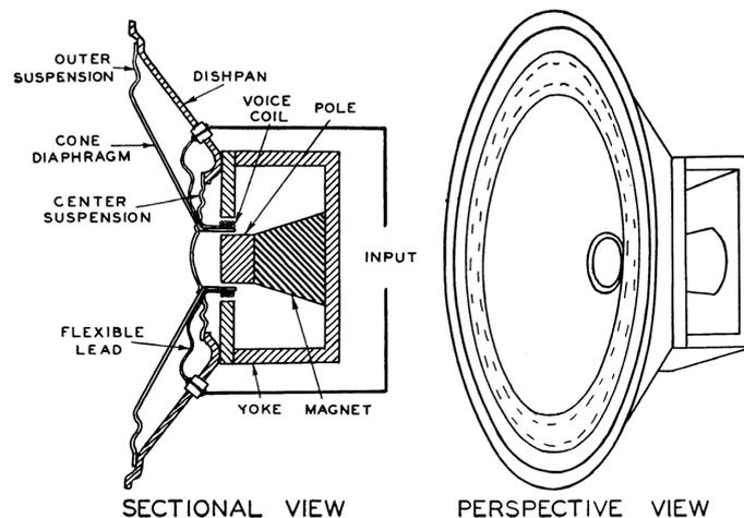
Figure 5.7: Permanent-magnet dynamic loudspeaker in cross-sectional and perspective views.
