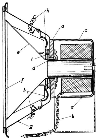
Figure 4.10: Cross-section of an electrodynamic loudspeaker.
