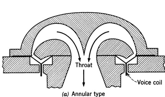
Figure 6.7: Drive system of a diaphragm.
