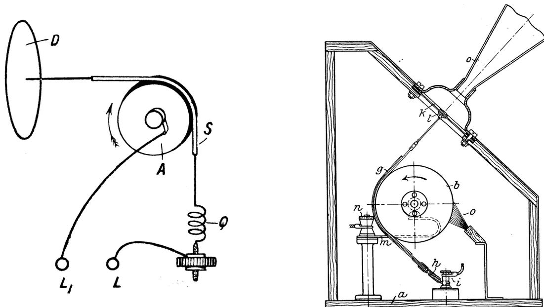
Figure 3.2: Principle and construction of a Johnson-Rahbek loudspeaker
