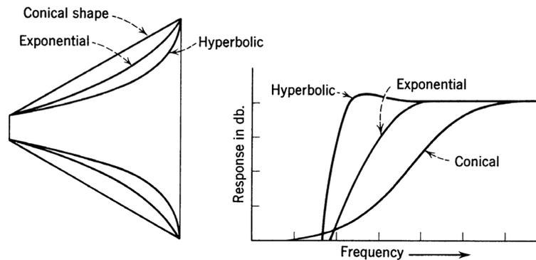
Figure 6.6: The low frequency cutoff of a horn-loudspeaker depends on it's shape.
