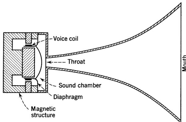
Figure 6.3: Basic components of a horn-loudspeaker.
