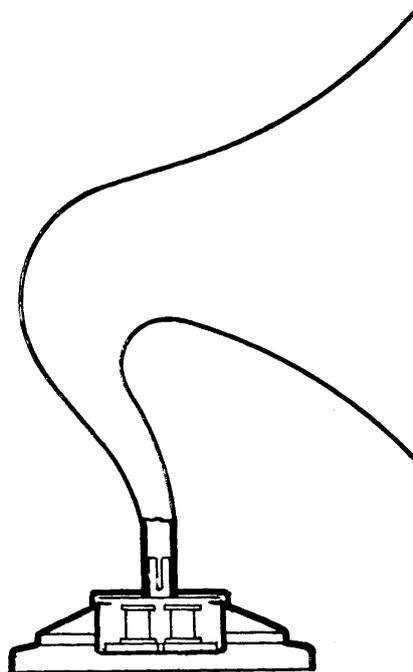
Figure 2.2: Typical horn-loudspeaker form.
