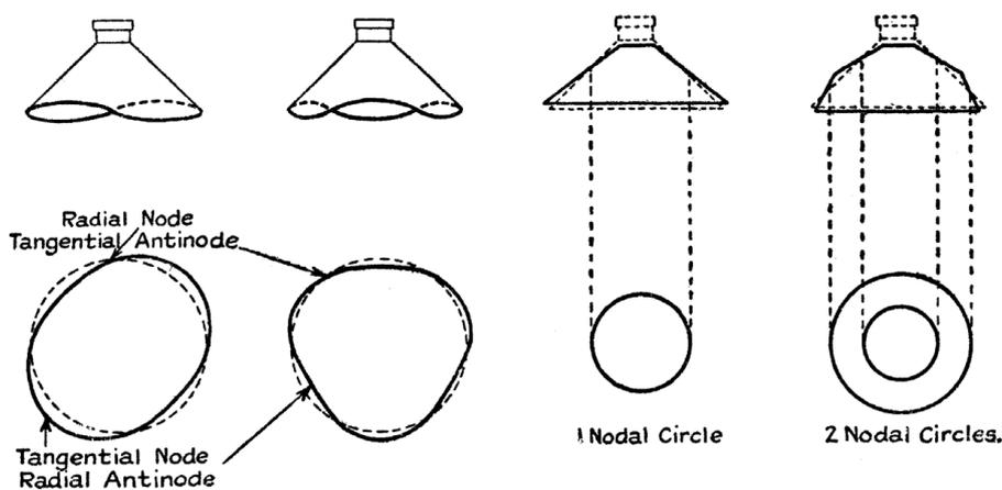
Figure 5.13: Examples of standing-waves which can develop in the diaphragm at high frequencies.
