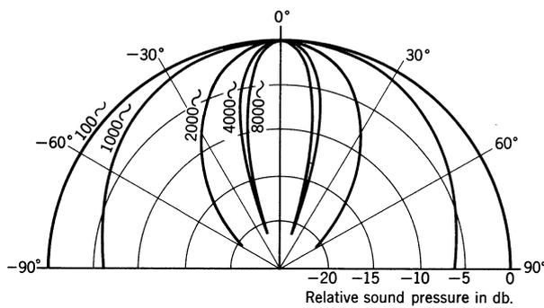
Figure 5.15: Example of the directivity of a loudspeaker as a function of frequency.
