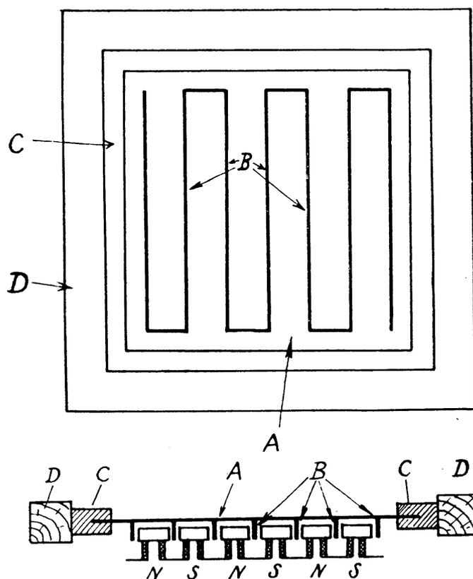
Figure 4.13: Principle of the leaf loudspeaker
