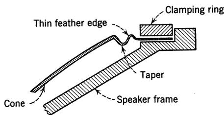
Figure 5.11: Outer attachment of the diaphragm; the bead runs softly so that the restoring force is minimized.
