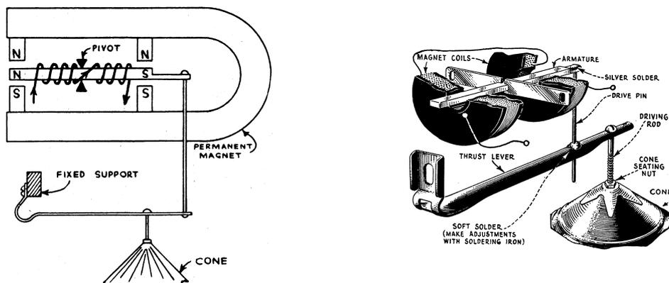
Figure 4.3: Four-pole system principle and perspective detail; The lever tilt is adjustable.
