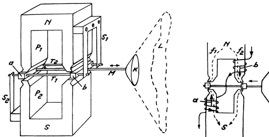
Figure 4.5: The inductor-dynamic system.
