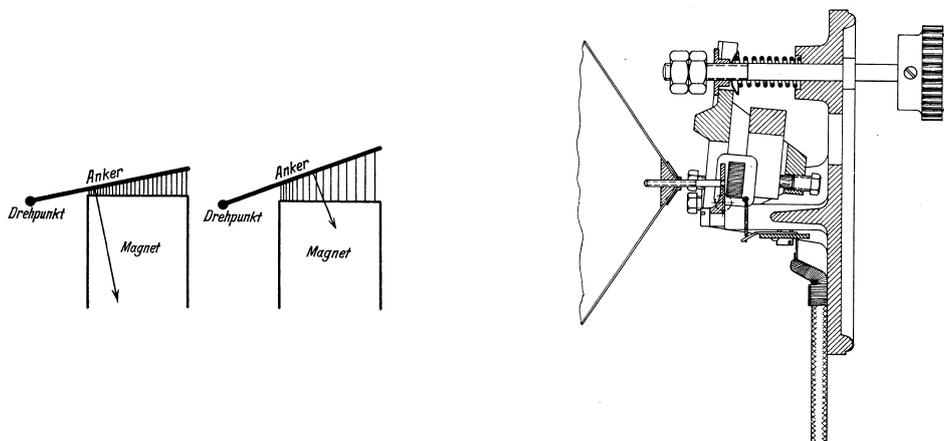
Figure 4.4: Principle and cross-section of the AEG Gealion loudspeaker with low frequency compensation
