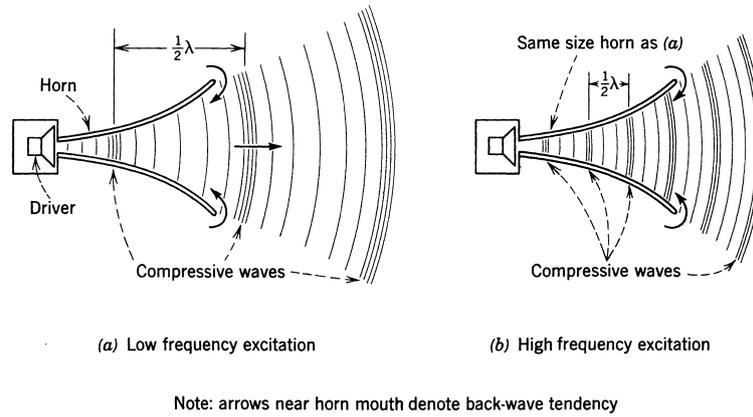
Figure 6.5: The lower frequency limit of a horn loudspeaker; At lower frequencies, which is to say at longer wave lengths, the reflected back wave (curved arrows) cancels the radiated wave, thereby decreasing volume.
