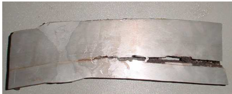
Figure 1 : Pictures of blisters and step-wise cracking due to HIC
