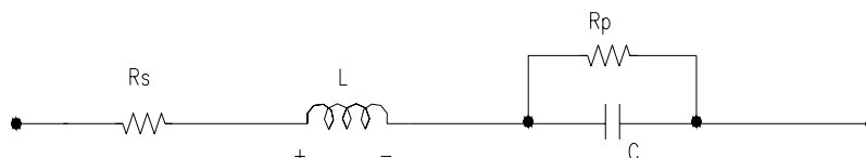
[Fig. 2] The first-order circuit model of an ultracapacitor. Each of four circuit elements is ideal.
