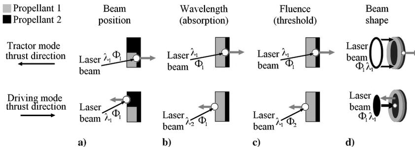
Fig. 2 Control parameters for direct targets (gray arrows indicate direction of ablation exhaust).
