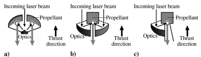
**Fig. 1 Conceptual diagrams, in cross section, of indirect laser propulsion tractor beam targets (gray arrows indicate direction of ablation exhaust).**
